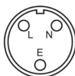
'Top Box' Power Female Connector (Connector polarity as seen from outside of 'Top Box')
